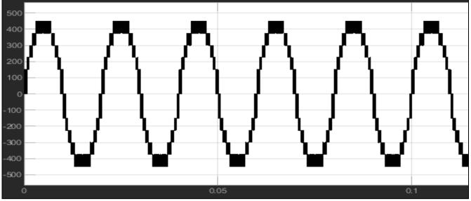
Fig.9. Output Voltage of Eleven Level Hybrid Multilevel Inverter with Reduced Switch Count
