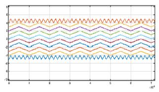
Fig.6 (a) Multi carrier signals for VF-PWM
