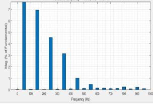
Fig.10. Frequency Spectrum of Output Voltage of PD-PWM
