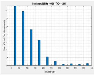
Fig.11 Frequency Spectrum of Output Voltage of POD-PWM
