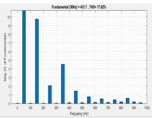
Fig.14 Frequency Spectrum of Output Voltage of VF-PWM
