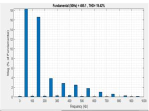
Fig.15 Frequency Spectrum of Output Voltage of Third Harmonic Injection –PWM
