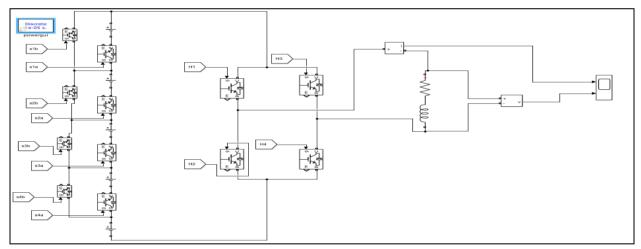
Fig.8 Simulink Model of Eleven Level Hybrid Multilevel Inverter with Reduced Switch Count
