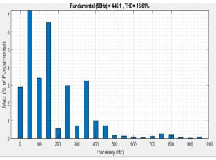
Fig.13 Frequency Spectrum of Output Voltage of CO-PWM
