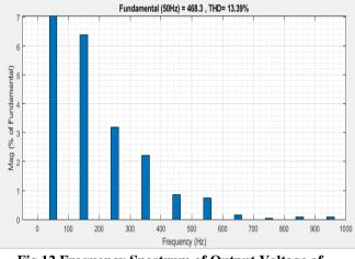
Fig.12 Frequency Spectrum of Output Voltage of APOD-PWM
