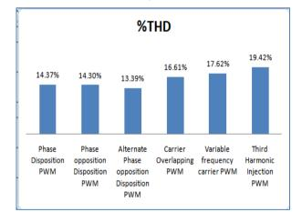
Fig.16 Graph of Different PWM Techniques versus % THD
