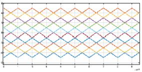
Fig.4 (a) Multi carrier signals for APOD-PWM
