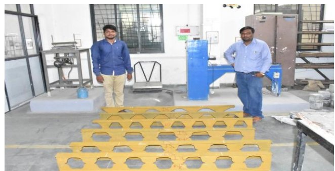
Fig. 8: Specimens of the castellated beam.
