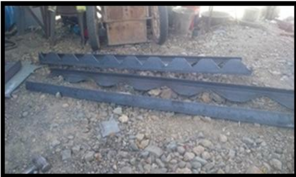
Fig.4. Separation and Rearrangement of two halves of section.
