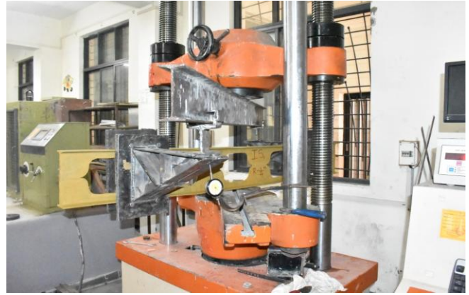
Fig. 6: Torsion Assembly of Castellated beams for Torsion Test.
