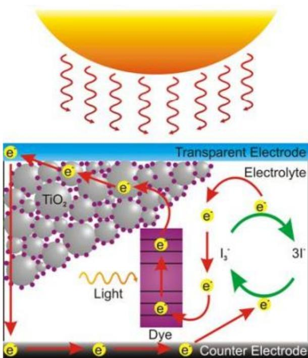
**Fig. 2.2: The mechanism of DSSC**
