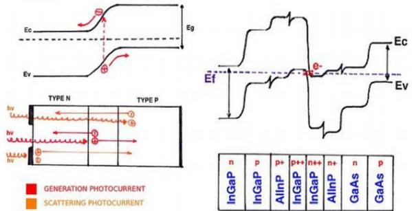
**Fig.2.3: Schematic illustration of the PV effect and band structure of the tunnel junction**
