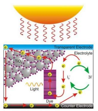
Fig. 2.2: The mechanism of DSSC
