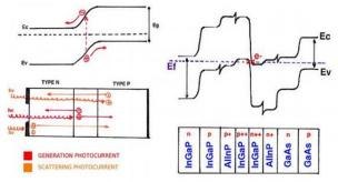
Fig.2.3: Schematic illustration of the PV effect and band structure of the tunnel junction
