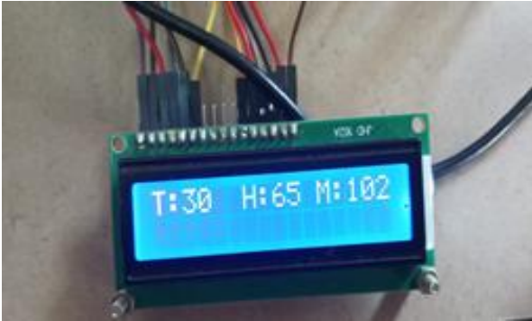
Figure 8(b): Output readings of Temperature Humidity and Moisture content of the soil
