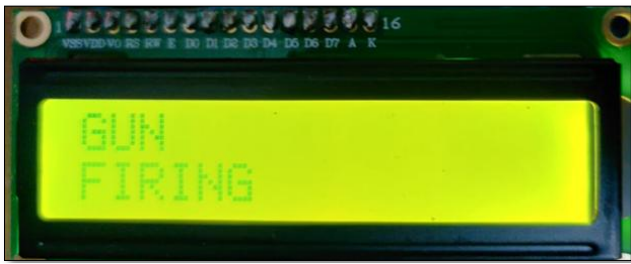
Figure 7. LCD on Intruder Detection due to Sensor
