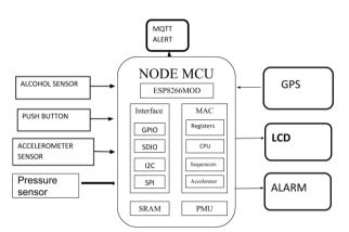
Fig.1- Block diagram of NODE MCU
