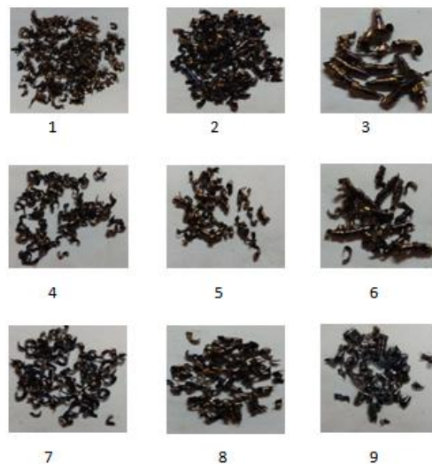
Fig. 6 Chips produced by carbide insert having chip breaking design.
