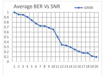
Fig. 2 Average BER Vs SNR for GMSK modulation.
