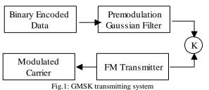
In GSM it is eminent that the Gaussian filter requires a normalized bandwidth i.e. product of bandwidth and symbol time (*BxT*) of 0.3 to avert inter-symbol interference (ISI). Also, it is been studied that to evaluate ISI, the interference of two adjacent bits is more than enough, which lies at either side of the currently processed bit. The gain *K*, shown in Figure 1 ensures that the modulation index  $\beta$  is explicitly maintained at 1/2 [16].
