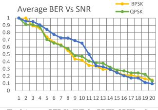
Fig. 3 Average BER Vs SNR for BPSK, QPSK and GMSK modulation.
