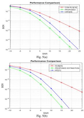
Fig. 5(a & b) Comparison between proposed and various methods for 5 users.
