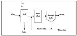
Fig. 4: Schematic of UASB
