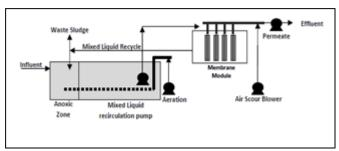
Fig.5: Schematic of MBR
