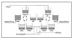
Fig. 3: Schematic of SBR
