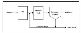
Fig. 1: Schematic of Initiated Sludge Process
