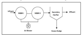
Fig. 2: Schematic of MBBR
