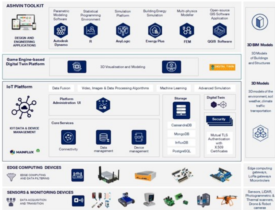
Figure 2: ASHVIN platform software architecture
