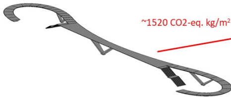
Figure 14 Carbon Footprint of the bridge in an early design phase
