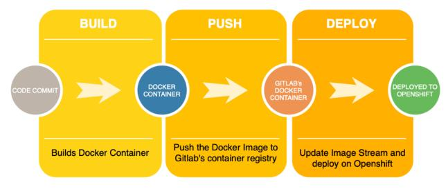
Fig. 2 CI/CD Pipeline for automatic redeployment
