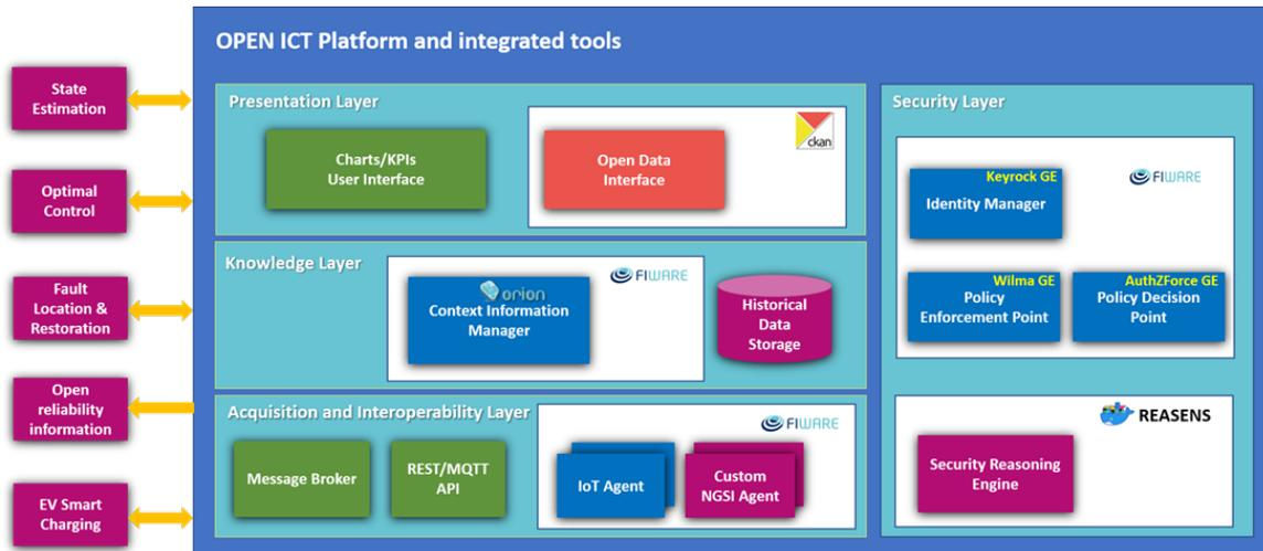
Figure 8: HYPERRIDE services using the Open ICT Platform.
