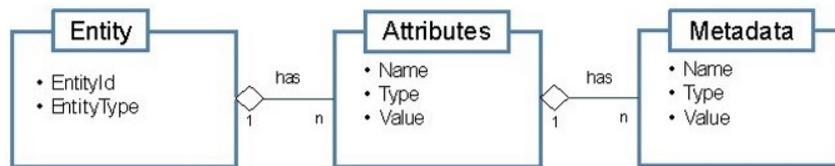
Figure 3: NGSi data model (FIWARE-NGSI v2 Specification, *n.d.*).
