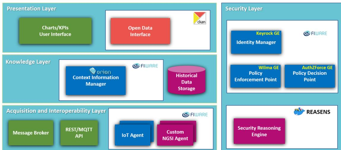
Figure 2: Overarching HYPERRIDE Open ICT Platform Architecture and Integrated Tools.
