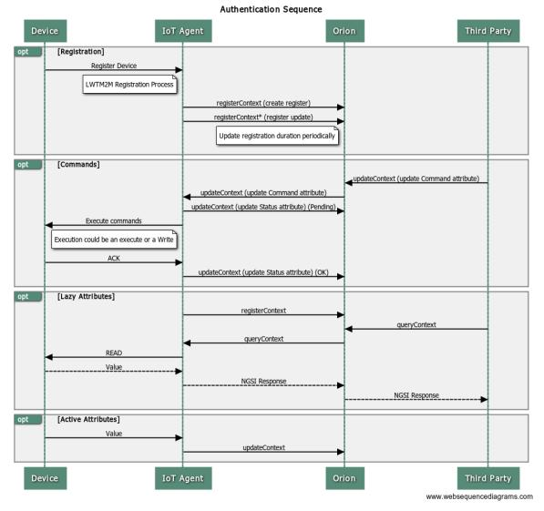
Figure 4: NGSI interactions of an IoT Agent with the context broker (iotagent-node-lib Architecture, n.d.).
