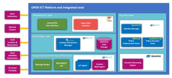
Figure 8: HYPERRIDE services using the Open ICT Platform.
