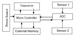
Figure .2 Sensor node's components
