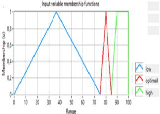
Figure:11 Humidity input variable with low, optimal and high membership functions
