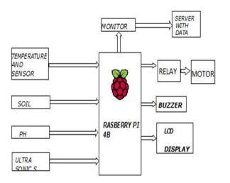
FIG 4. Block diagram of IOT Based automatic crop field monitoring
