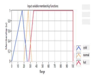
Figure 10: Temperature input variable with cold, normal and hot membership functions
