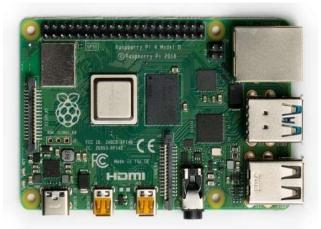
Fig 2. Raspberry pi 4 model b
