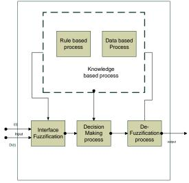
Figure 7. The block diagram of fuzzy logic controller
