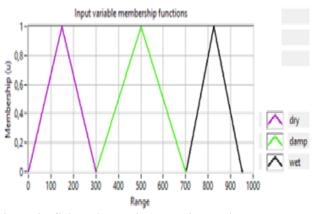
Figure 8: Soil moisture input variable with dry, damp and wet membership functions
