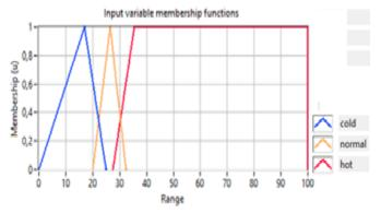
Figure 9: Temperature input variable with cold, normal and hot membership functions membership function of the temperature input variable. The orange triangle in Figure 4..16 represents a "normal" membership function of the temperature input variable with temperatures
