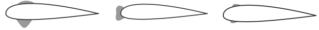
FIG 6. Schematic illustration of different artificial wing ice shapes; left: run-back ice, mid: leading-edge ice, right: SLD-ice configuration
