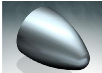
Fig. 2 CAD of the spherically blunted tangent ogive nose
