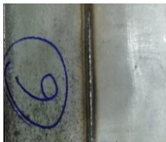
Fig 2: Macrograph of Laser Welded Sample
