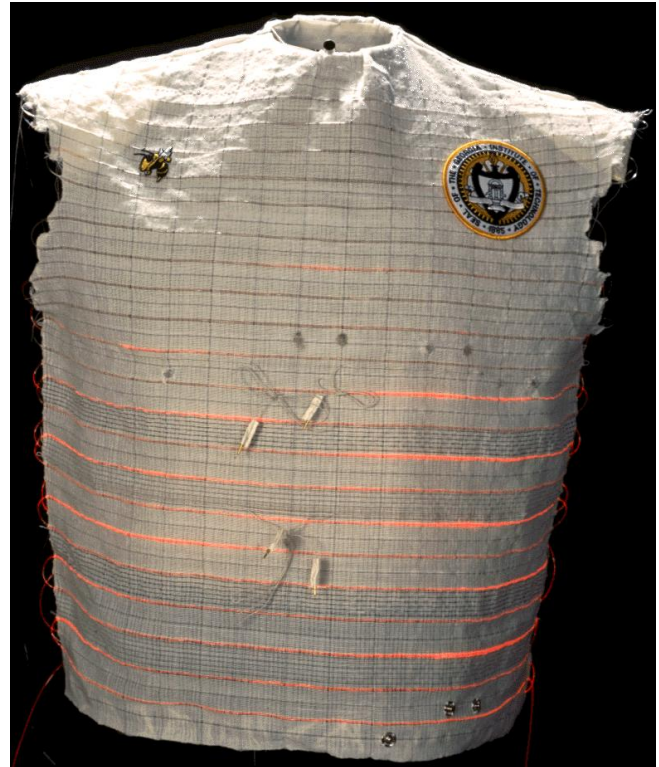
Fig. 6. The "Wearable Motherboard," or Smart Shirt, developed by the Georgia Institute of Technology, features a single plastic optical fiber spirally integrated into the fabric with a novel weaving process to eliminate discontinuities at the armholes or seams.
