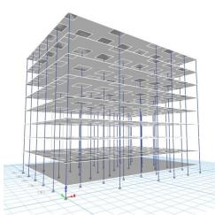
Fig. 5. Isometric view for Flat slab building in ETABS.
