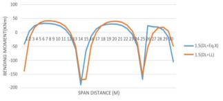
Fig. 9. For flat slab 1.5(DL+Eq.X) with 1.5(DL+LL) for R=2.
