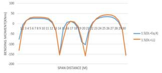
Fig. 11. For flat slab 1.5(DL+Eq.X) with 1.5(DL+LL) for R=4.
