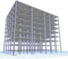
Fig. 6. Model 3D view for Flat slab building in ETABS.
