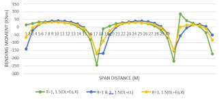
For flat slab 1.5(DL+Eq.X) with 1.5(DL+LL) **Fig. 14**. for R=1 Vs R=3.
