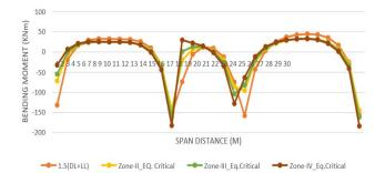
Fig. 17. For flat slab 1.5(DL+Eq.X) with 1.5(DL+LL) for R=5, Zone-II, III, IV.
