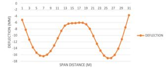
Fig. 18. For flat slab deflection Vs span dist. For R-3 & zone-II.
