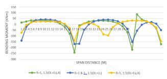
Fig. 15. For flat slab 1.5(DL+Eq.X) with 1.5(DL+LL) for R=1 Vs R=5.
