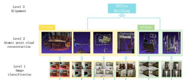
Fig 3. Annotated hierarchical SfM approach workflow
