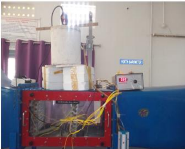
Fig 7 Double heat exchanger (series connection)
