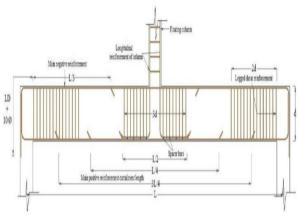
Fig.2. Transfer beam which support Floating Column
