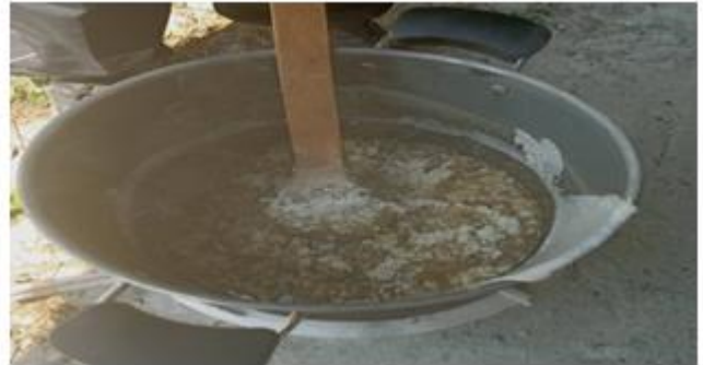
Figure 3. Mixing of melted wastes with sand
