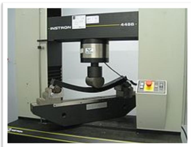
Fig.10. Universal Testing Machine (three-point fixture)
