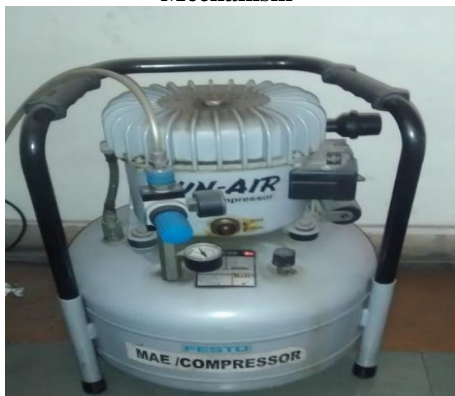
Fig.6 Used Compressor with attached buffer tank
