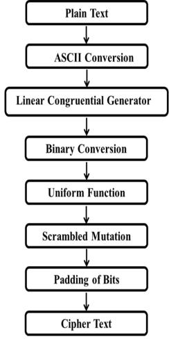
Fig.4. Overview of Encryption Process
