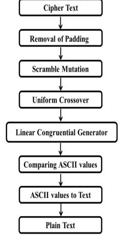
Fig. 5. Block Diagram of Decryption Process
