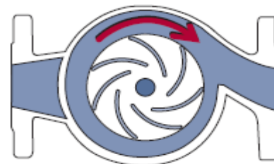
Fig 6 – Liquid Flow through impeller
