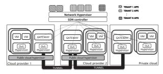
Fig. 1: Network virtualization architecture
