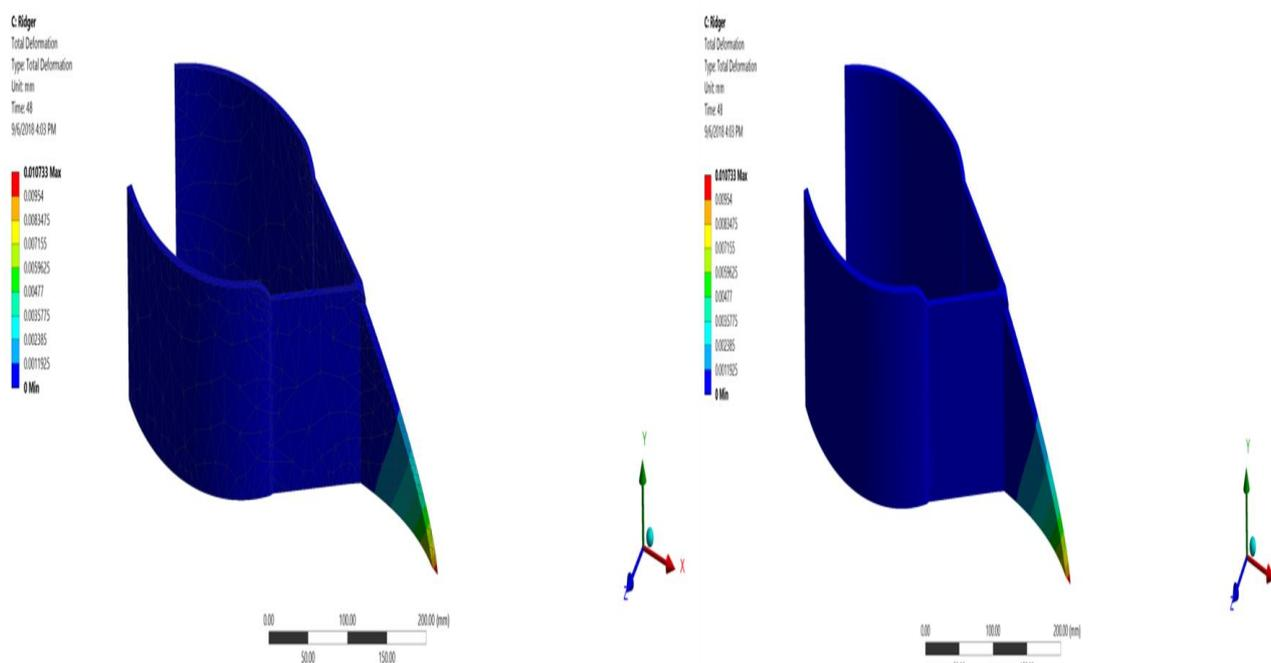
Fig. 6a. Total deformation (meshed) contour plot- ridger bottom, 6b) Total deformation contour plot
