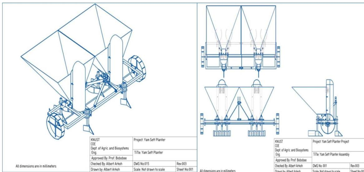
Fig. 9a: Planter Pictorial Drawing; 9b, Planter 3<sup>rd</sup> Angle Projection
