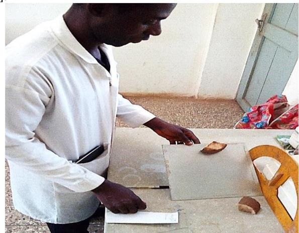
Fig.1: Angle of repose determination
