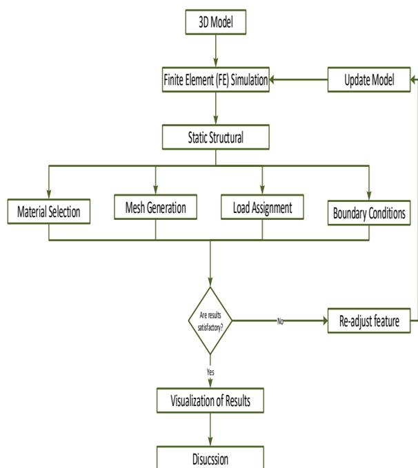
Fig 2: FEM simulation setup flow
