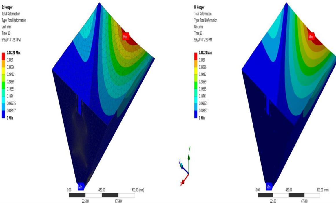
**Fig. 4a. Total deformation (meshed) contour plot- hopper, b) Total deformation contour plot**
