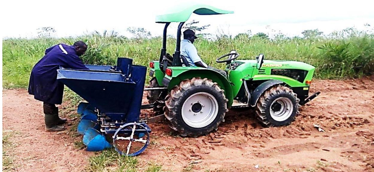
Fig. 10: DRMM planter Hitch to Category I Tractor during field trials
