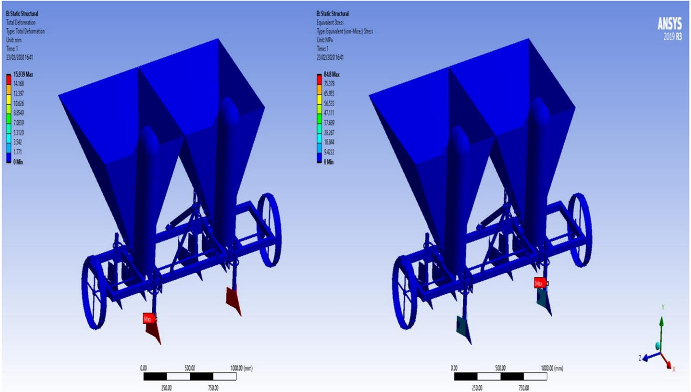
Fig. 7a. Total deformation,
