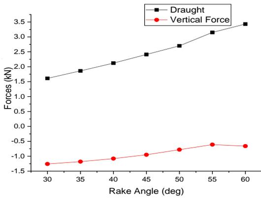
**Fig. 3: Effect of rake angle on draught and vertical force**
