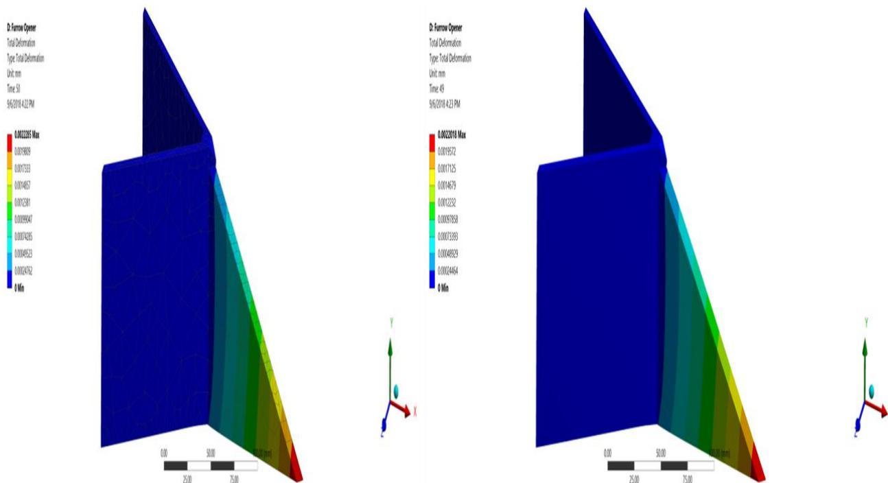
Fig. 5a. Total deformation (meshed) contour plot- furrow opener, 5b) Total deformation contour plot
