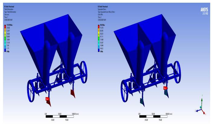
Fig. 7a. Total deformation,
