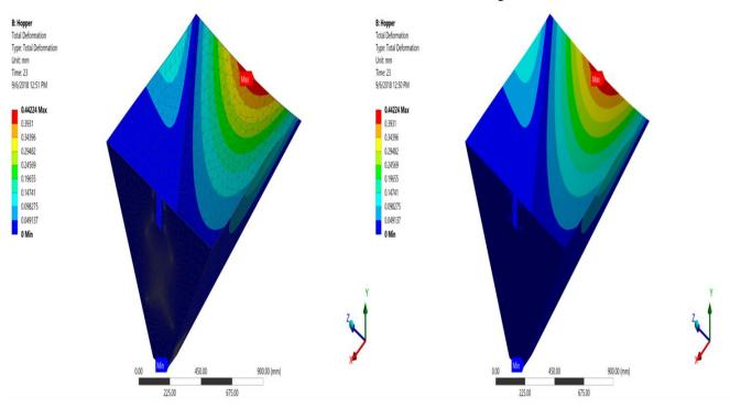
Fig. 4a. Total deformation (meshed) contour plot- hopper, b) Total deformation contour plot
