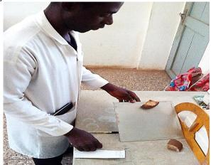
Fig.1: Angle of repose determination
