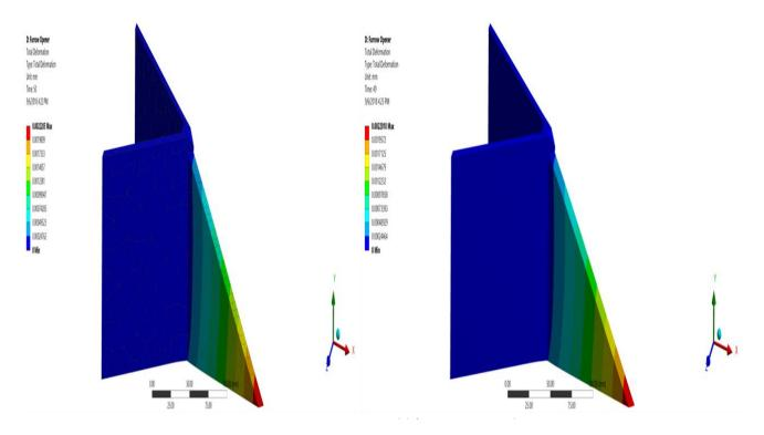
Fig. 5a. Total deformation (meshed) contour plot- furrow opener, 5b) Total deformation contour plot
