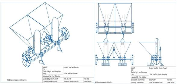
Fig. 9a: Planter Pictorial Drawing; 9b, Planter 3rd Angle Projection
