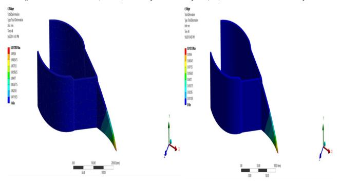
Fig. 6a. Total deformation (meshed) contour plot- ridger bottom, 6b) Total deformation contour plot
