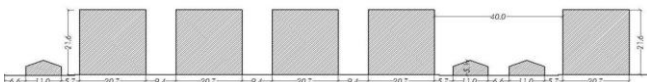
Fig. 8: Section of the model area of the base case with H/W ratio of 0.54 in E-W direction [3].
