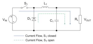
Fig.1 Buck Converter [13]
