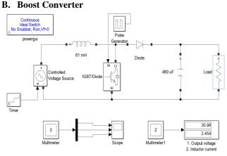
Fig.20 Boost Convertor - open loop
