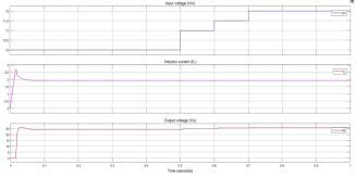
Fig.24 Simulation results for Boost Converter in Closed loop with variable input
