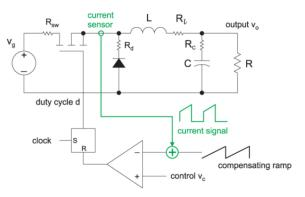
**Fig.3 Buck Converter current control loop** [1] The DC gain for the current mode buck converter is:
