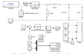
Fig.17 Buck Convertor – Closed loop
