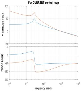
Fig.14 Effect of input voltage variation on the Control **Characteristic of the Boost Converter**
