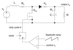
Fig.5 Boost Converter voltage control mode [1]
