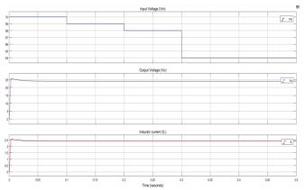
Fig.19 Simulation results for Buck Converter in Closed loop with variable input
