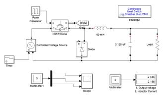
Fig.15 Buck Convertor – open loop
