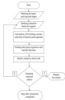
Fig.12 Flowchart for modeling of the converter
