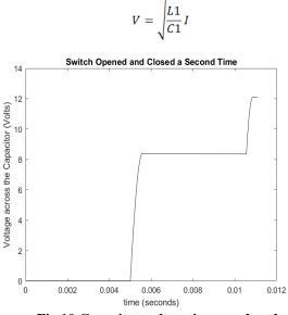
Fig.10 Capacitor voltage in second cycle
