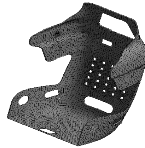
Figure 3 Meshed model of racing seat
