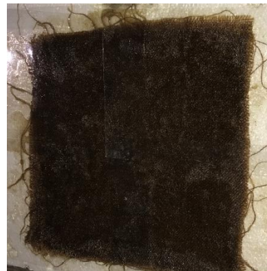
Fig. 5. Jute fiber with mud crab shell powder
