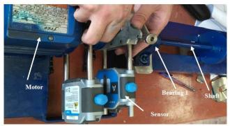
Fig. 11Measuring misalignment in horizontal direction.
