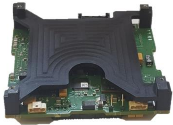
Figure 2. 1 TB storage for Space. RC64 serves as the storage controller. Several 3D NAND flash devices make the highly protected, high endurance storage
