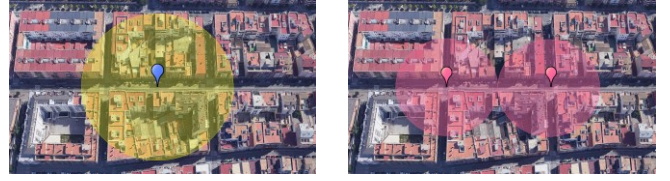
Fig. 4. Map of the geographical area served by the EVS service, featuring two intersections and including an IEEE802.11p RSU: one EVS instance and corresponding covered intersections highlighted in yellow (left), two EVS instances and corresponding covered intersections highlighted in pink (right)
