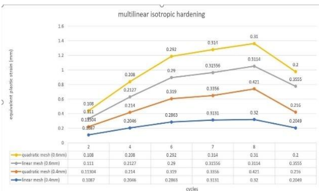
Figure 24. linear and quadratic element type with 0.4mm and 0.6mm mesh size, multi-linear isotropic hardening
