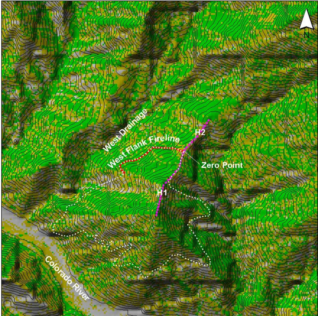
**Figure 25. Fuel model map at 10 meter resolution for the South Canyon Fire vicinity. FM 10 - dark green; FM 4 - green; FM 2 - tan; FM 99 (barren-rock) - gray. Lines and notation shown are described in Figure 23.**
