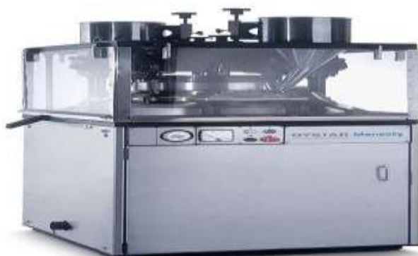
Fig.9:-Double sided bi-layer tablet press
