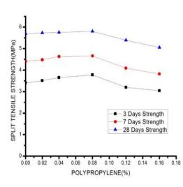
Figure 4: variation of split tensile strength with polypropylene fibres
