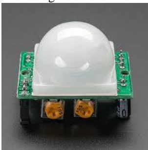
Figure (b) Passive Infrared Radiation Sensor
