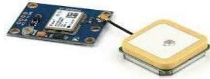
Figure (c) NEO 6m GPS module
