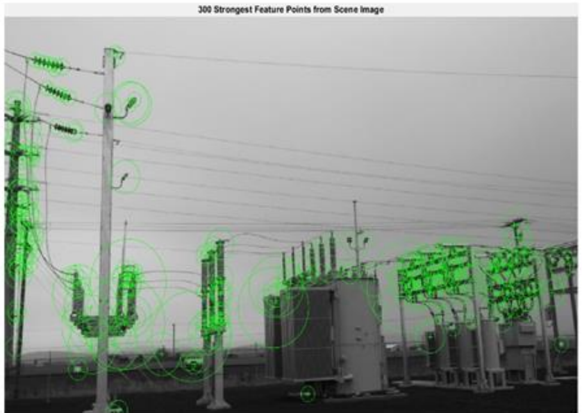
Fig. 9 50 strongest features in insulator image Fig.10 300 strongest feature points of scene image
