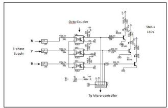
Figure 2 Circuit diagram of Phase Sequence Detection Circuit
