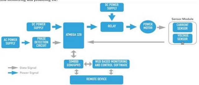
Figure 1 Block Diagram of proposed Model
