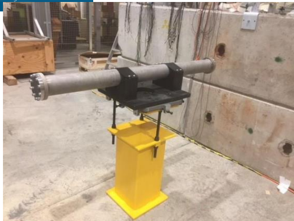
Small-scale replica of the SHiP target
