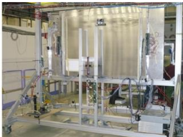
Prototype of MRPC (HS timing detector)
