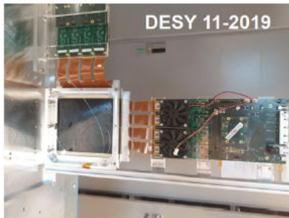
Prototype of a scintillating fibre module of the SND target tracker
