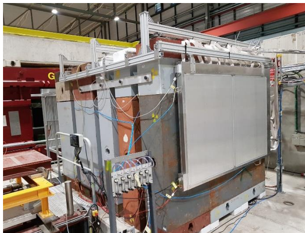
Prototype of the SND muon ID system
