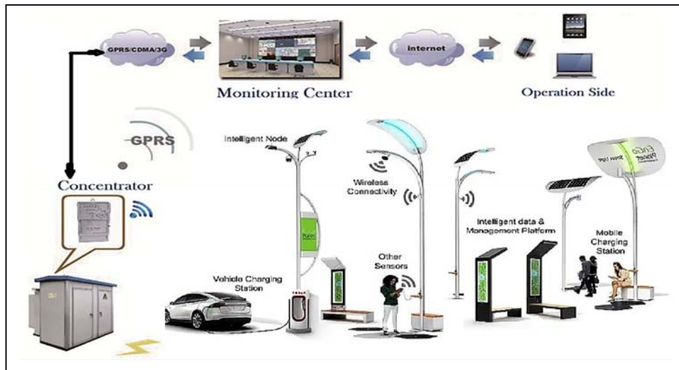
Fig. 2: Typical Smart Street Lighting for Smart City (Source: lightingindia.in, gaoterled.com)
