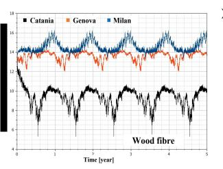
If compared with the saturation moisture content (w<sub>sat</sub>), the TWC in the CLT corresponds – in Genova and Milan – to slightly less than 15% of the maximum moisture content, and slightly exceeds the w<sub>80</sub>
