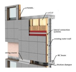
e-CLT integrates both local bio-based recyclable (or recycled) insulating materials and customizable cladding finishing solutions. Size and number of CLT panels to be applied on the façade are determined based on the initial seismic deficiency of the building and the assumed target performance
