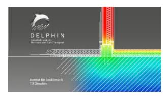
DELPHIN 6.1 is a software tool developed at University of Dresden that allows a detailed 2-D numerical study of the dynamic heat and mass transfer phenomena inside building components, including vapour diffusion, vapour and liquid sorption and capillary suction
