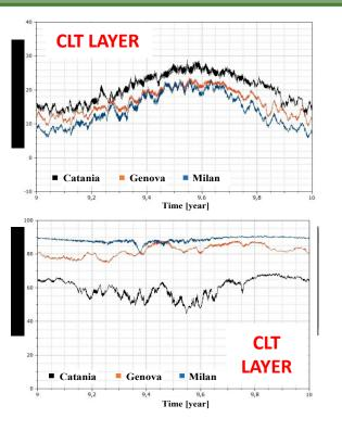
There is a remarkable difference amongst the selected climates, especially when looking at relative humidity values (RH) occurring inside the wooden materials (CLT and fibre)
